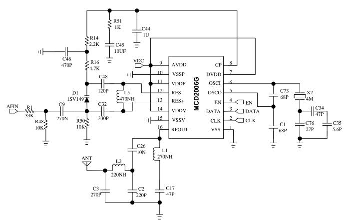
■ For MCD2006T 49.840MHz with  $50\Omega$  output impedance matching:
