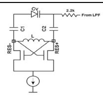
The setup of the VCO can be summarized as follows. Firstly, open the loop, build up an oscillation (as shown in above picture). Two capacitors connected at pin RES- and RES+ are recommended as 100~120pF (when loop locked at 49MHz). The inductor connected between pin RES- and RES+ need to be calculated according to following equation.
